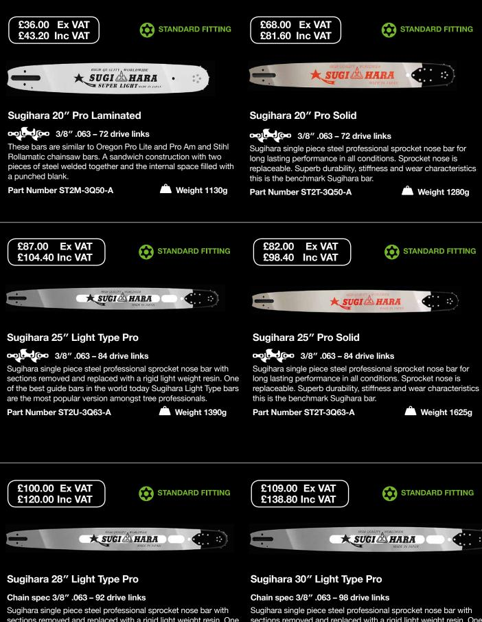
Sugihara single piece steel professional sprocket nose bar with sections removed and replaced with a rigid light weight resin. One of the best guide bars in the world today Sugihara Light Type bars are the most popular version amongst tree professionals.
