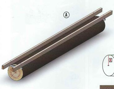
**Step 1:** Arrange first cut guide on log (fig A). Slabbing bracket system is shown, but principle is similar if using EZ Rails. For best results, measure the distance from the center growth ring (X) on the narrow end, and mark corresponding distance on wide end of the log (fig C). Set mill on first cut guide as shown (fig B). Starting from the wide end, begin your first cut. The first cut will look like a wedge (fig C)
